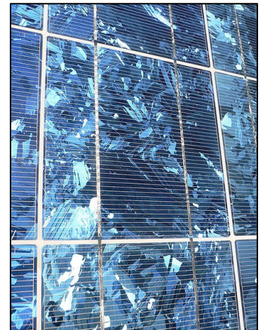
Figure 15. Polycrystalline Solar Cell
